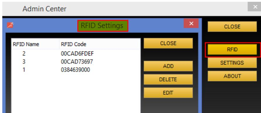
To load new RFID chips into the system, the entire Tendo Sprint System must be connected to a computer, and the RFID chip reader must be attached to a photocell.
