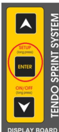
•Long press (press and hold) of the Setup button (middle button - ENTER) will activate the setup menu of the external display
