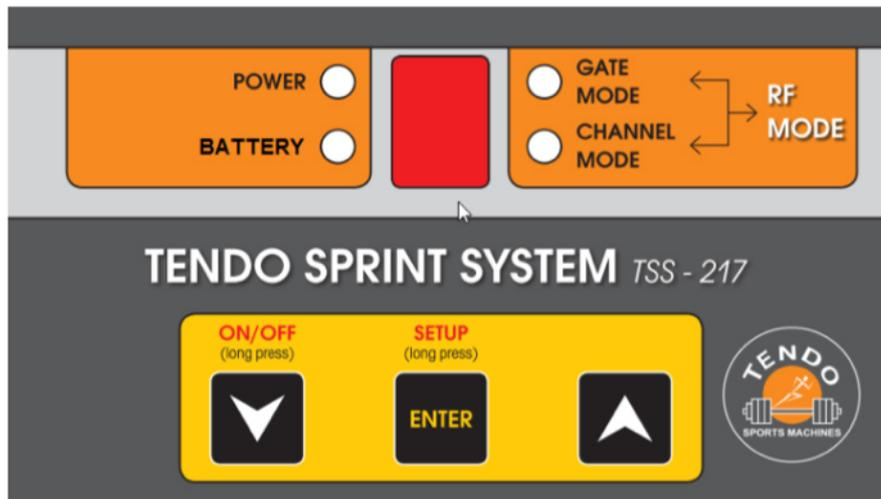
Immediately after the ON/OFF button is released, information about a current setting of the photocell is shown on a LED display for 5 seconds.
